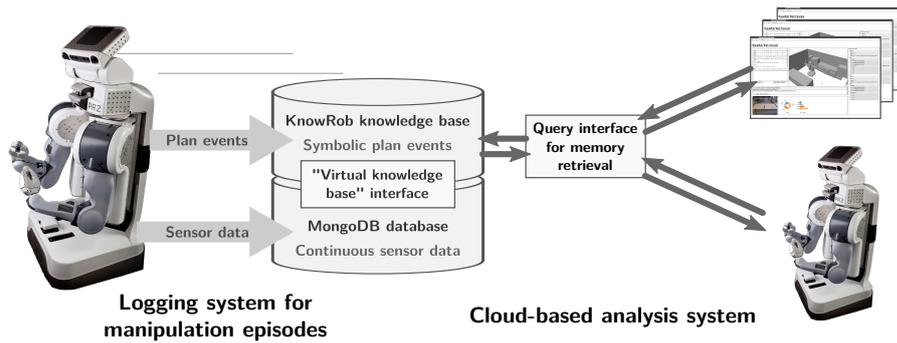
Fig. 2: Overview of the OPEN-EASE system. The logging components record detailed log data of manipulation episodes into a knowledge base. A library of query predicates is provided for reasoning about the data and can be called by human or robot clients via the Internet.
