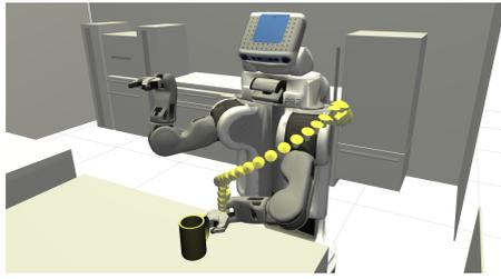
Fig. 3: Memorized grasping trajectory for picking up a cup
